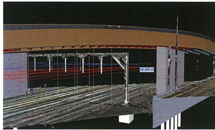
BRIDGE SOUTH ELEVATION (EAST TRACKS) - APPROX CLEARANCE 10.245 M TRACK TO BRIDGE BEAM
